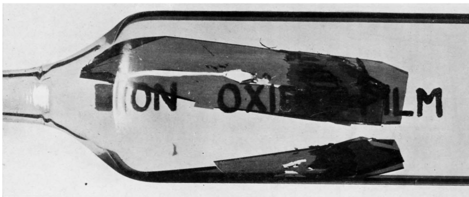
Stripped film (from blue heat-tinted iron) in reaction tube. (Legend beneath shows transparency of film, except where folded.) ( \times 1\frac{1}{2} .)
